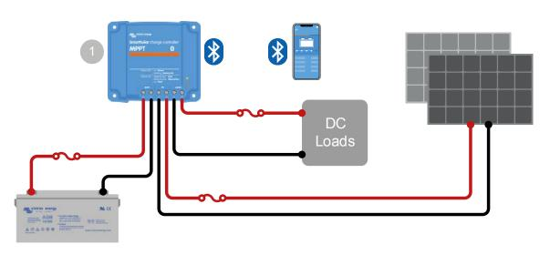
Solar charger with a load output. The load output protects the battery against a too deep discharge.
