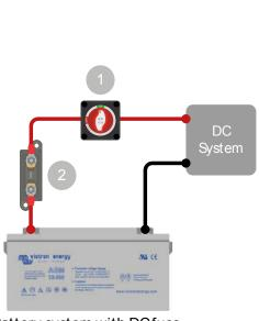
Battery system with DC fuse, DC battery switch and DC loads.
