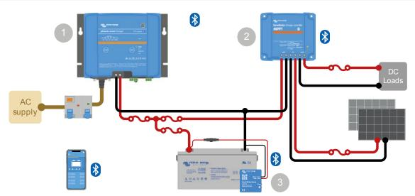
The Smart Battery Sense sends battery temperature and voltage information via Bluetooth and the VE Smart Network to the solar charger and the AC charger and is used for temperature and voltage compensated charging.
