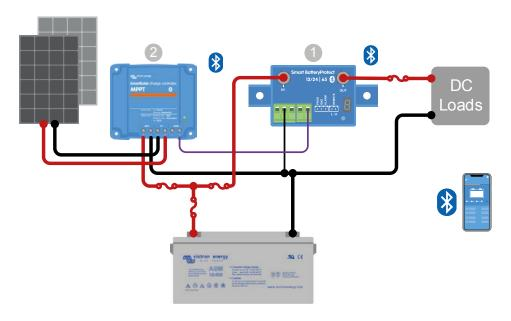
System with a small solar charger. The BatteryProtect is used to increase the load output current rating of the solar charger.
