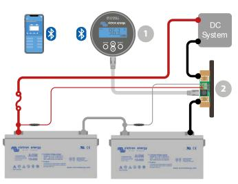
System with a BMV-712 Smart battery monitor. The battery bank is monitored and the auxiliary connection is used to monitor the battery bank midpoint.
