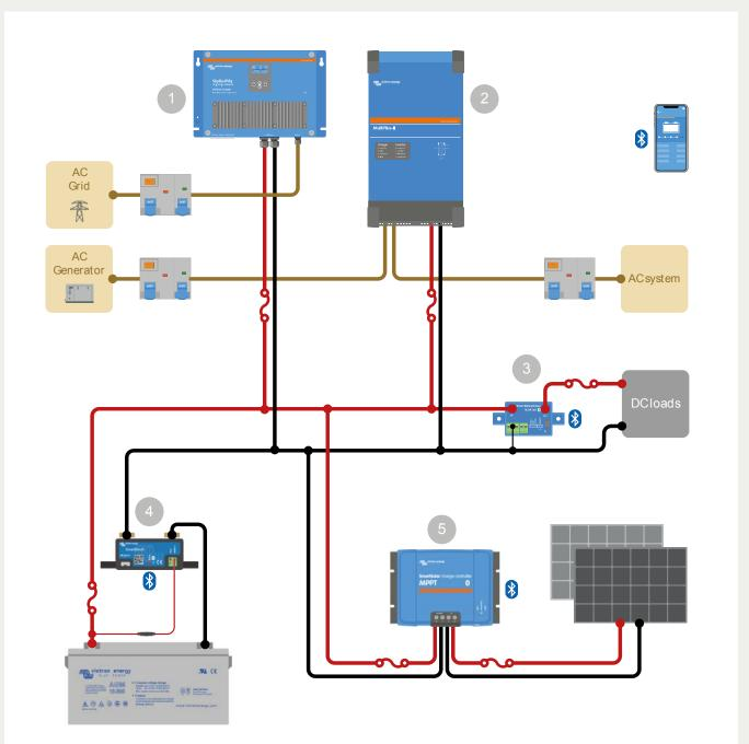
Inverter system decoupled from the grid, use when the grid is unsuitable as an input for an inverter/charger.
