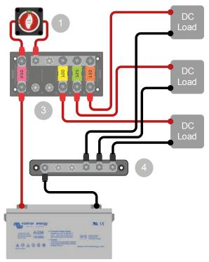
Battery system with Busbar, fuse box and DCloads
