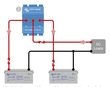
The Argodiode battery combiner combines two battery banks to supply a single DCload circuit. For example for use in DC backup systems.
