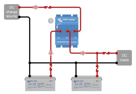
The Argodiode or Argofet battery isolator allows multiple battery banks to be charged from one charge source.
