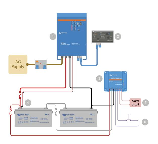
System with a Skylla battery charger and a battery balancer. The battery balancer ensures that both batteries in a 24V system are charged equally.
