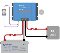
System with DC-DC converter, providing galvanic isolation between the battery and the DC load or circuit.
