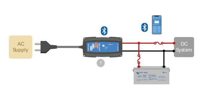
Battery charger used to charge a battery and providing power to DCloads.
